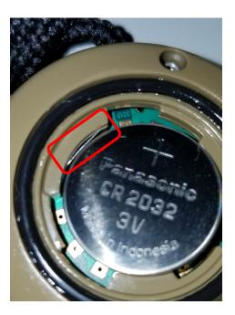
2) The side of the battery needs to make contact with this battery clip as shown above.
