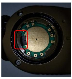
3) If the clip was pushed down so it is flat against the board below (see above), the battery will sit on top of the clip and not work. Gently use tweezers to push the battery clip back into position so the side of the battery can make contact again. Or send it in to us for repair.
