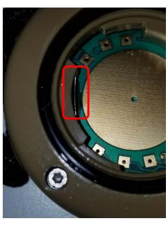
1) Locate the battery clip inside the battery cavity. It looks like a rectangular piece of silver metal that should be perpendicular to the board below and up against the plastic post behind it.
