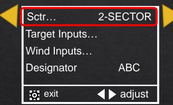
To scroll between different sectors, highlight Sctr... and press the left or right buttons.
