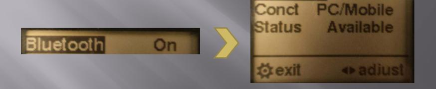
Please note: If Status is showing as Connected, the Kestrel may already be connected to a different device. You will need to close this connection before connecting with this new device. You can toggle Bluetooth to OFF and then back to ON to help close this connection.
